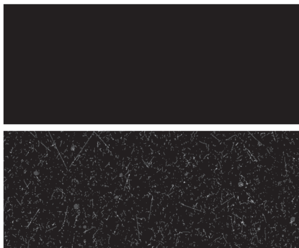
Figure 3: Absence of readout noise and dark current in PILATUS Hybrid Photon Counting detectors.
